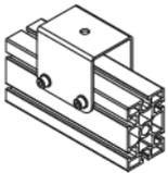
**NOTE:** The left and the right anchoring points have to be fixed at the same distance from each end side of the cabinet.
